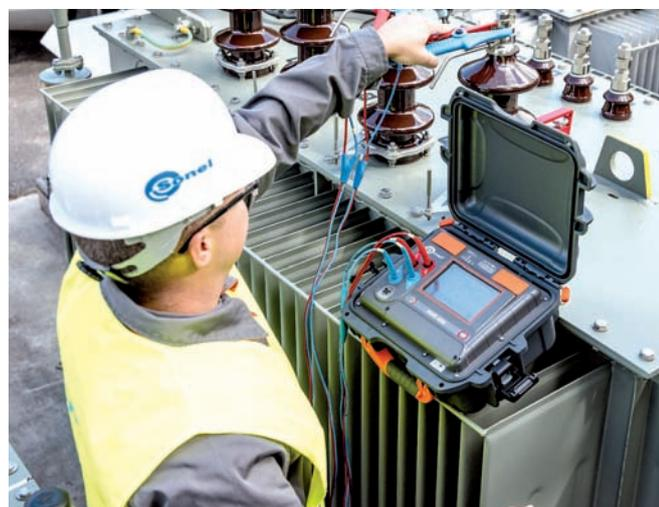
Measuring transformer winding resistance with the SONEL MMR-650.
