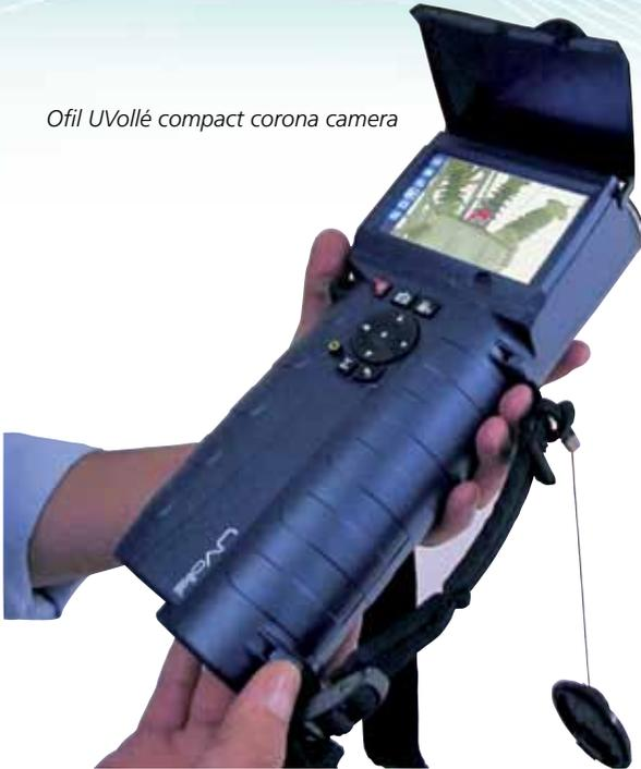
Infrared and Ultraviolet inspection technologies are being used to assess the condition of operating electrical components and installations. Infrared thermography detects temperature changes and is proportional to the square of the current drawn. In the absence of current no heat develops, regardless of voltage.
