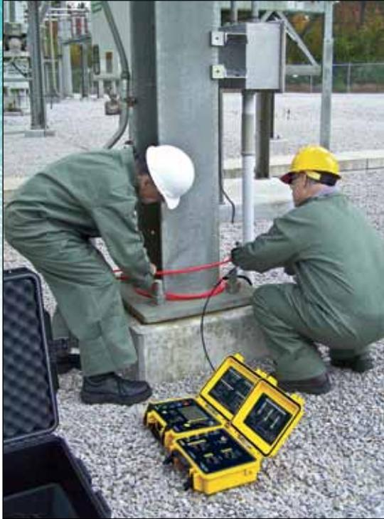
*AEMC GroundFlex used to measure the earth resistance of a structure*
