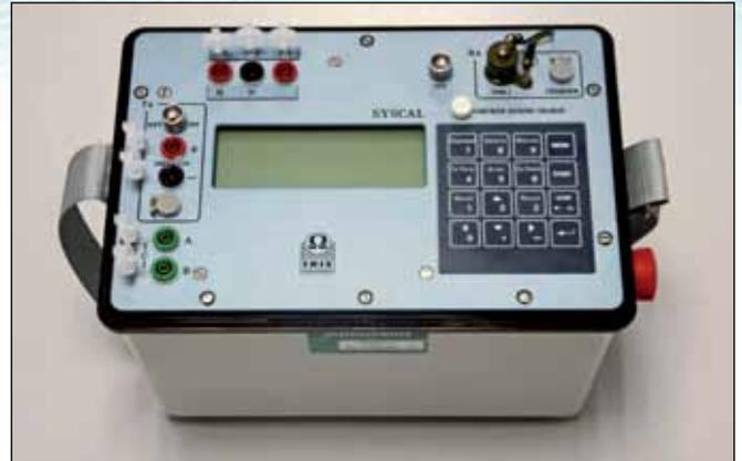
*Syscal's Soil Resistivity instrument*
